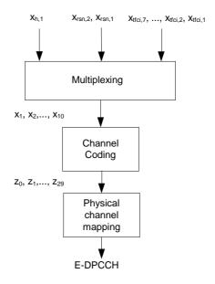
Figure 23: Coding chain for E-DPCCH
